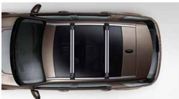
Roof Rails* VPLCR0137 – Silver finish (panoramic roof) VPLCR0133 – Silver finish (fixed roof)** VPLCR0136 – Black finish (panoramic roof) VPLCR0132 – Black finish (fixed roof)** Roof rails facilitate easy fitment of cross bars for roof carrying. Pre-set positioning points ensure cross bars are fixed in optimum position for weight distribution and dynamics. Maximum payload is 75 kg.†
